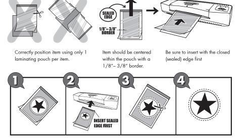
For smaller or irregular shaped items, position item in center of adequate pouch and trim after lamination. DO NOT CUT LAMINATING POUCH TO FIT ITEM BEFORE LAMINATION.
