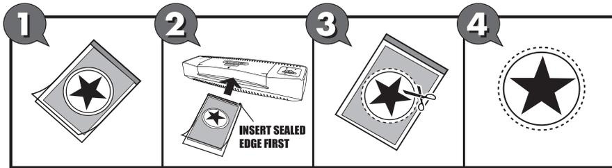
**For smaller or irregular shaped items**, position item in center of adequate pouch and trim after lamination. **DO NOT CUT LAMINATING POUCH TO FIT ITEM BEFORE LAMINATION.**
